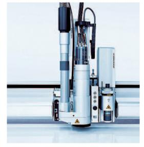
For great results in nonferrous materials, Zund offers an optional Minimal Quantity Lubrication (MQL) which applies a very small amount of lubricant directly onto the router bit. Technical Committee's opinion:
